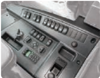
Centralized Instrument switch Panel
