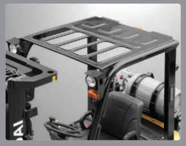
**Strong overhead guard** The safety overhead guard meets ISO 6055 regulations and protects the operator during hazardous jobs.
