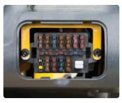
An accessible, compact fuse box for easy inspection
