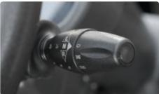
**Multi-function switch lever** A multi-functional switch lever gives easy access to lights and horn.
