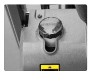
**Brake fluid reservoir** Highly visible and accessible reservoir makes daily inspections a quick and easy job.
