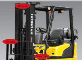
**OPSS (Operator Presence Sensing System)** Control of mast tilting, lifting and lowering is not possible when the operator is not in the normal position.
