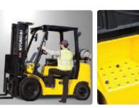
Large footstep & Handle Wide "open"step ensures easy and safe access to the operator's seat
