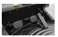
**Ergonomic positioned pedals** Based on human engineering, the accelerator, brake and inching pedals are optimally positioned for operator's convenience. Easy to remove cleanable rubber floor mat.
