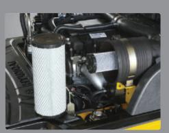
**Easy change air cleaner** The air filter is readily accessible for cleaning or replacement.
