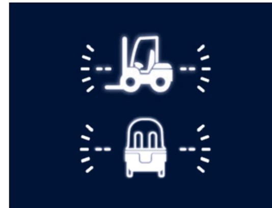
While driving the machine-control-unit (MCU) senses longitudinal and lateral movement and **alerts the driver if the preset stability values are exceeded.**
