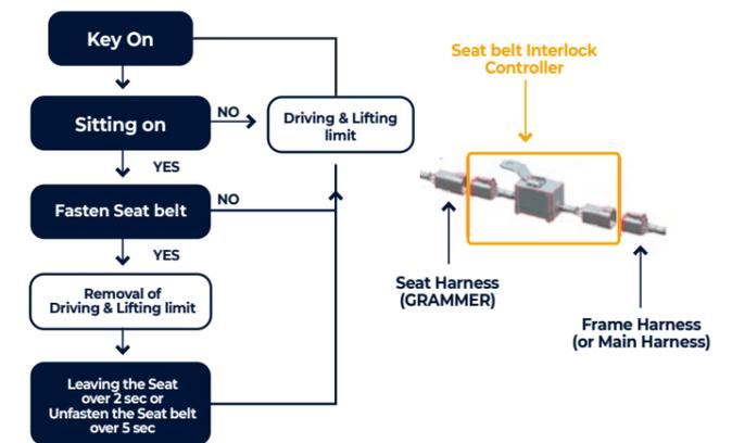
The seat belt interlock system protects operators from injury by **restricting equipment** operation if the seat belt warning has not been observed or if the operator unfastens the seat belt while driving.
